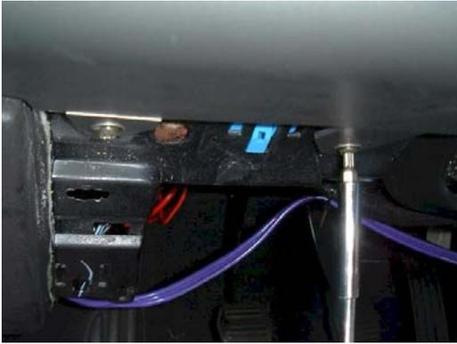
Remove the Torx Screw inside of where the 4 button console came out of
