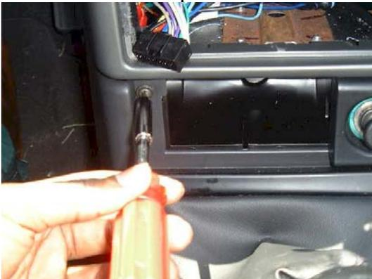
At this point you should be able to pull the Headlight Knob/dimmer Dash Piece and the Piece to the right of the steering wheel, its a large piece and doesn't need to come completely off. but far enough to allow access to the next set of torx screws
