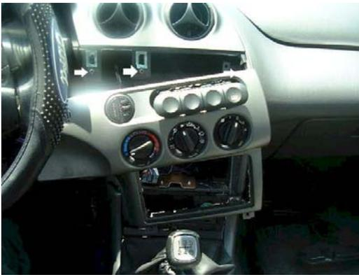
Remove the 2 Torx Screws from the stereo opening(on the upper edge- no photo)
